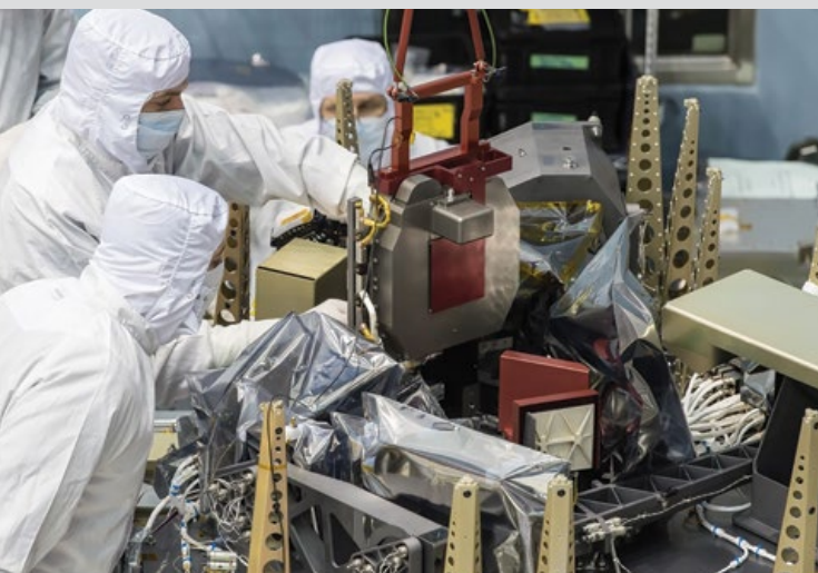
New Micro-Shutter Assembly being installed on the NIRSpec instrument by Airbus Defence & Space engineers (NASA/C. Gunn)
