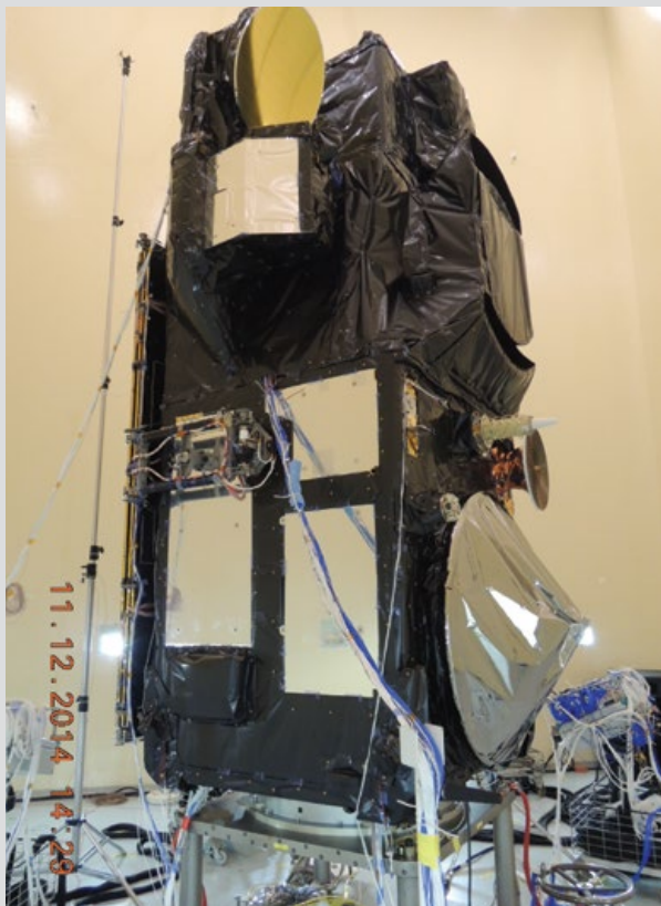
Sentinel-3A in the acoustic chamber at Thales Alenia Space France in Cannes (Thales)
