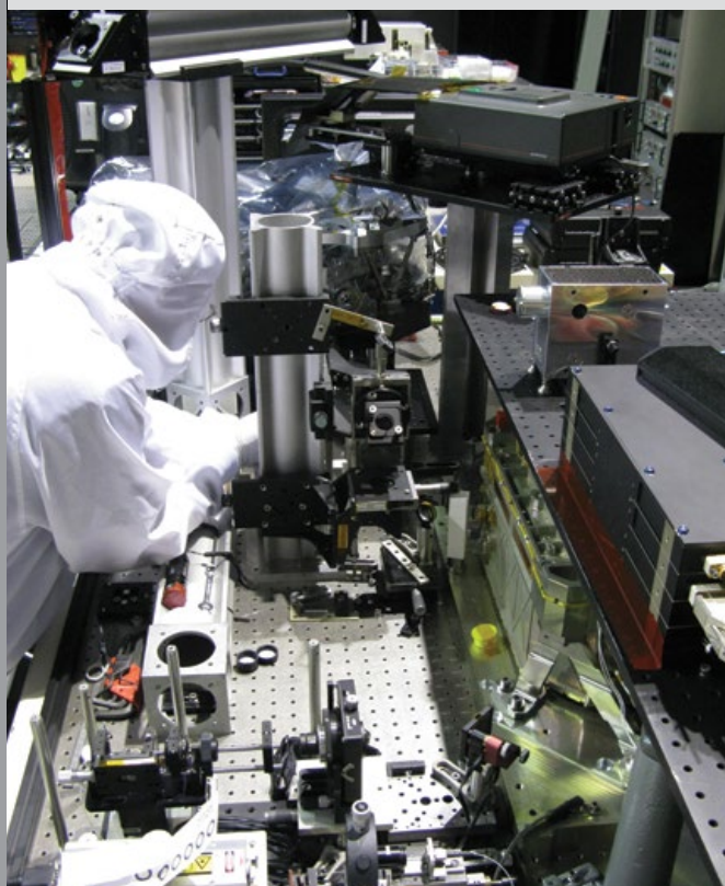
ADM-Aeolus alignment for Optical Bench Assembly Fluence Test (Airbus Defence & Space)
