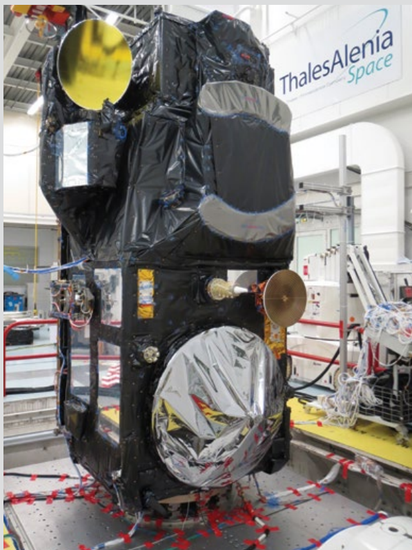
Sentinel-3A on the shaker at Thales Alenia Space France in Cannes ready for Sine Vibration test (Thales)
