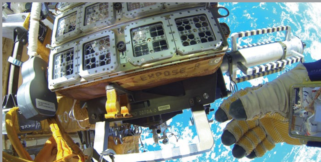
The Expose-R2 facility being installed on the ISS during a Russian spacewalk (Roscosmos)
