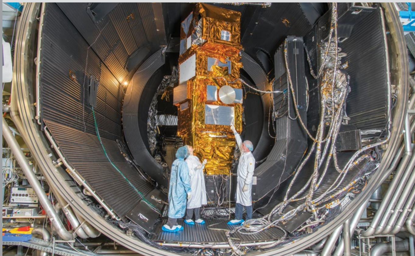
Sentinel-2A in the thermal vacuum chamber (Airbus Defence & Space/IABG)
