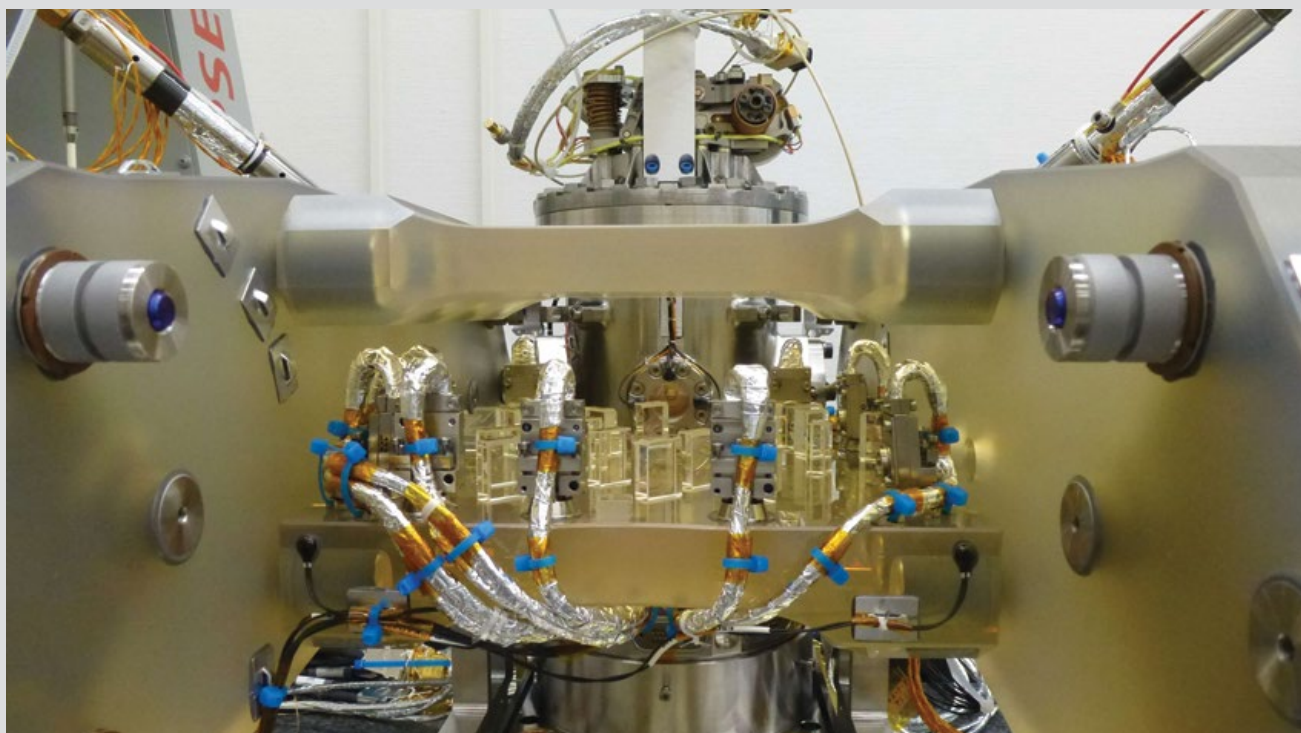
The LTP Core Assembly is ready to accept the Inertial Sensor Heads. In the background, ISH-1 with its window and the gold/platinum test mass in the centre. In front, inserts where ISH-2 will be aligned and fixed (Airbus D&S)
